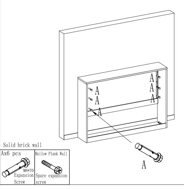
The first step, is to take marks on the wall, using impact drill tool to make holes, fix the bed frame on the wall with expansion screws
